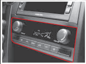
Heater/AC Control Panel
