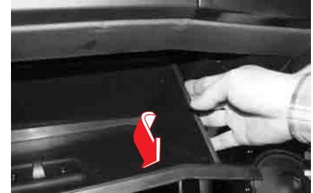
3. Push down the right side of the glove box in the direction of the arrow.
